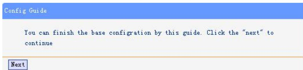
When press 'next', you can configure the Network parameters for the phone,
